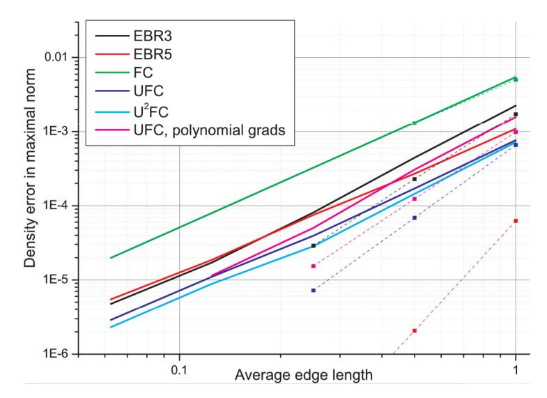
Solution convergence on triangular meshes: unstructured mesh versus TS-mesh (of the same color in dash)
