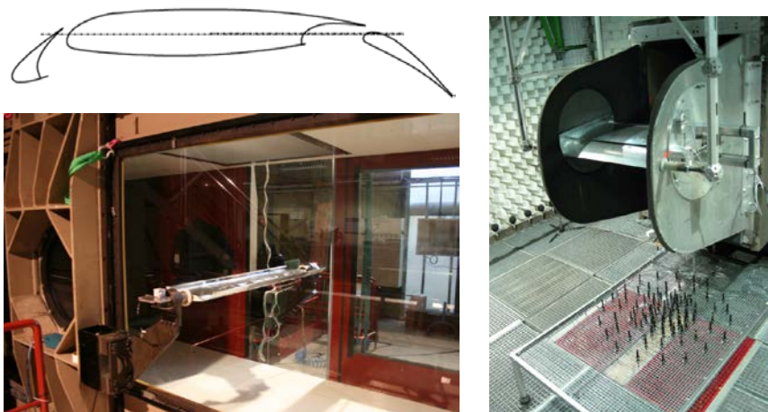
Fig. 1. Top left : F16 airfoil section. Model in F2 (left) and AWB (right)
