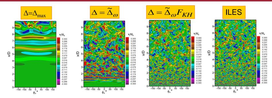
Contours of radial velocity on grid surface passing through nozzle edge
