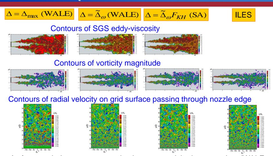
• As far as turbulence representation is concerned, both approaches (WALE with  $\Delta = \widetilde{\Delta}_{\omega}$  and SA with  $\Delta = \widetilde{\Delta}_{\omega} F_{KH}$ ) are close to each other, tangibly better than WALE DDES with  $\Delta = \Delta_{\max}$  and are nearly equivalent to ILES 28
