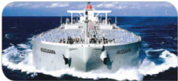
One of the largest means of transportation on earth: Malacca type VLCC ISUZUGAWA. 333m long and a loading weight of approx. 300,000 tons.
