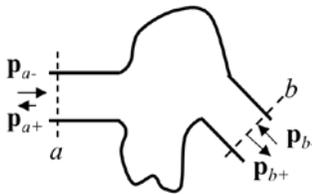
**Figure 1** A ducted multi-port with two openings  $a$  and  $b$ .
